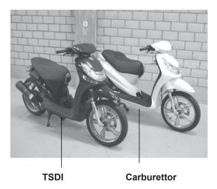
The Peugeot TSDI-System uses crankshaft driven air compressor. Gasoline is injected in the pressurised air of the feed rail where the premixing of air and fuel takes place. The air injector controls the admission of the rich mixture in the combustion chamber. The lubrication oil is dosed in the intake air of the engine by means of the oil pump.
