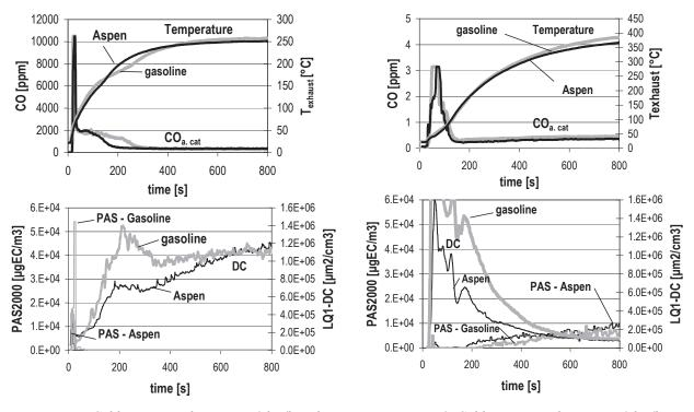
Fig. 7. Cold start - acceleration - 40 km/h with: Gasoline - Aspen, Peugeot TSDI Carb., oil: Panolin TS
