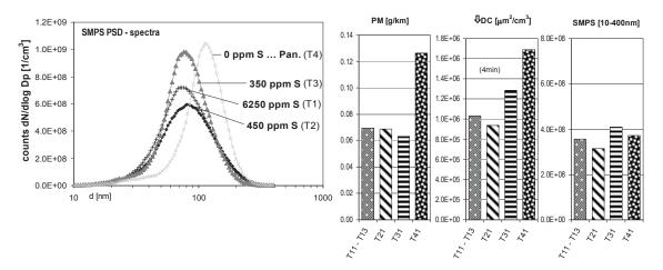
Fig. 9. Particle mass and nanoparticles at 40 km/h warm with gasoline and different lube oils, Peugeot Looxor TSDI
